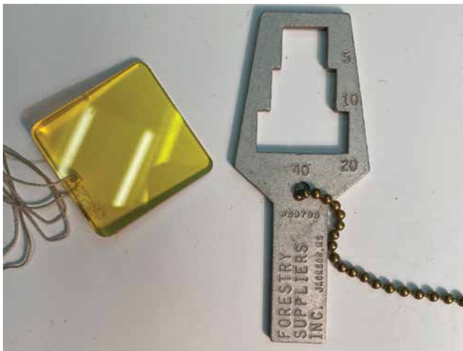
A wedge prism on the left, and angle gauge on the right, are forestry tools that determine basal area in variable plot sampling.
