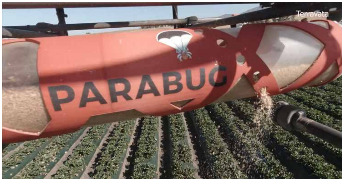
Predator mites are released from a cylinder attached to a drone. These mites prey on spider mites, a pest that can be detrimental to a farmer's crops. Submitted photos
