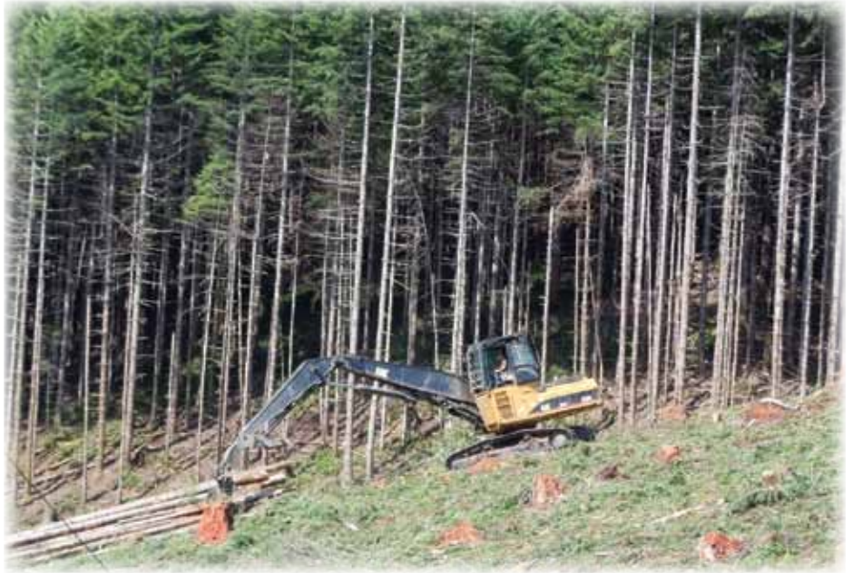
Shovel logging using tracked loaders is an excellent practice to reduce soil impacts.
