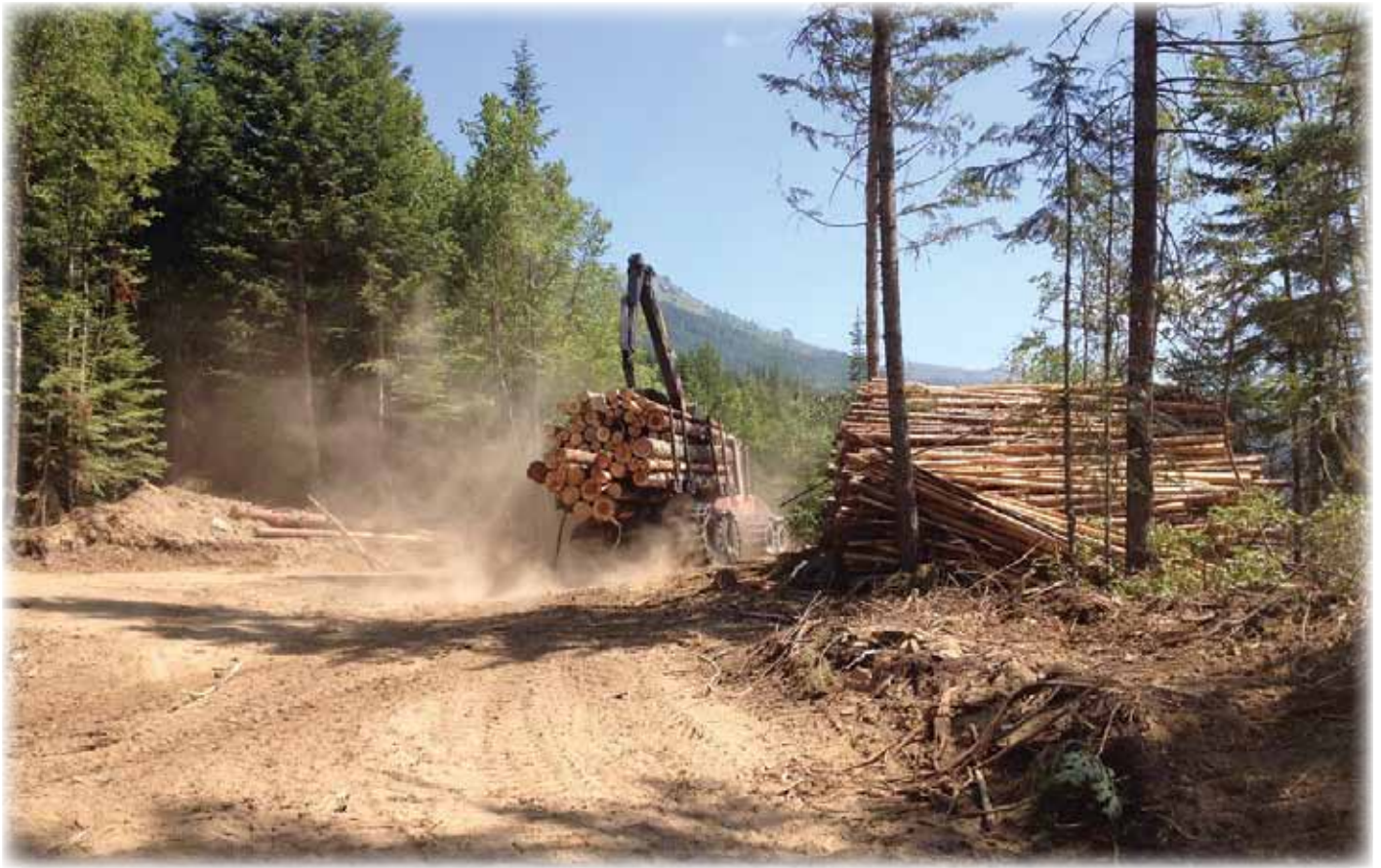
Ground based skidding can be obtained with self-loading forwarders.
