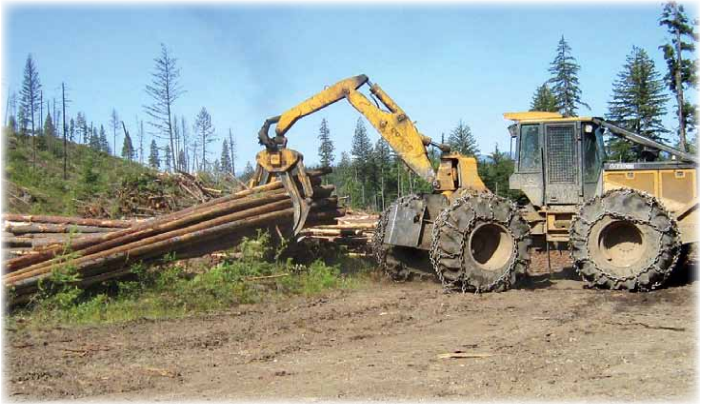
Ground based skidding using a grapple skidder. Machines can have rubber tires or tracks.
