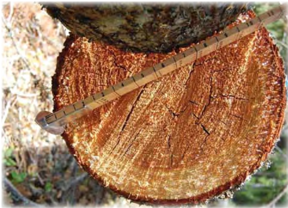
Logs are scaled based on diameter inside bark, shown, as well as length. If length and diameter are known, volume can be determined. This log diameter is about 10.5 inches inside bark.
