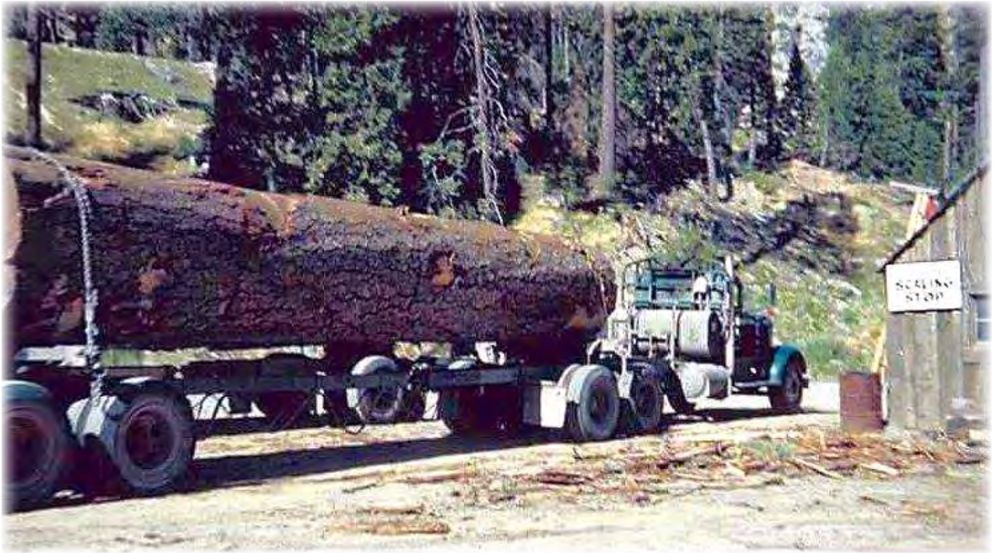
Logs can also be scaled by weight. Here a log truck is driving over scales to be weighed with logs loaded.
