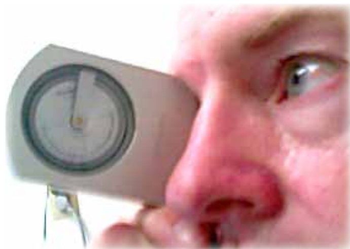
Using a clinometer to measure tree height. Note scale on the dial height.
