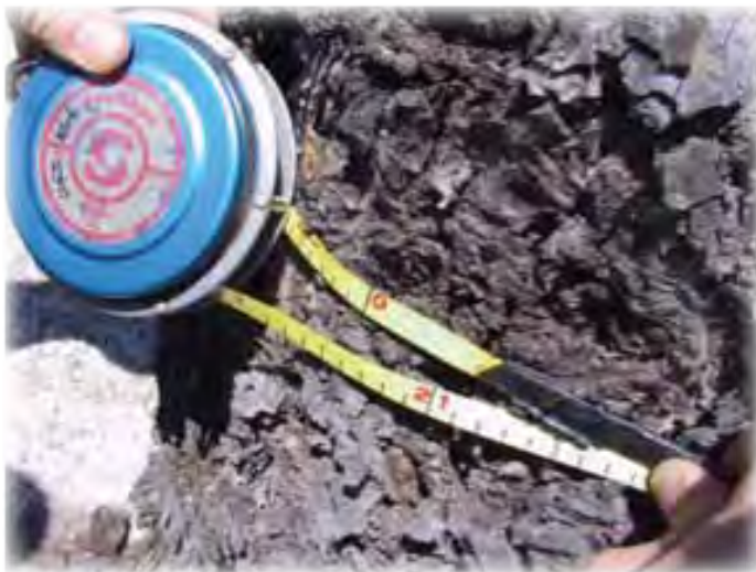
A diameter tape converts tree circumference to diameter in inches. This tree is 21.5 inches in diameter.
