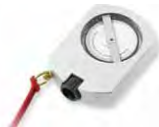
Using a clinometer to measure tree height. Note scale on the dial height.
